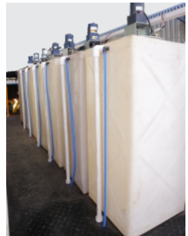
200 L SELF COLOR TANK ALONG WITH STIRRER
